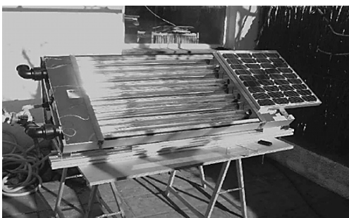
Fig. 1. SOLWATER and AQUACAT autonomous solar photoreactor prototype for water potabilization.
